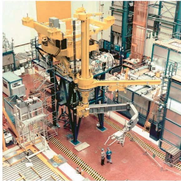
FIG. 11.61. Photograph of JET's Telescopic Articulated Remote Mast (TARM), equipped with a MASCOT manipulator.
