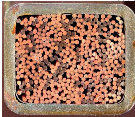
FIG. 5.20. The JT-60SA TF CICC 25.7 kA, 5.65 T, 18 \times 22 mm 2 (cable) (Courtesy of JT-60SA Ref. 5.8 ).
