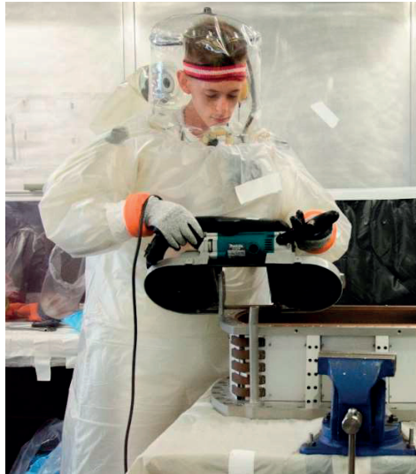
FIG. 11.39. Full PPE suit used for JET manual maintenance operations.
