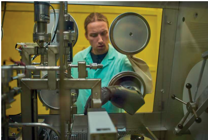
FIG. 10.13. Tritium confinement: Tritium is handled in primary systems (mainly made out of metal) which are installed in so-called secondary containments (mainly glovebox systems). Courtesy F. Priester, KIT.
