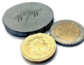
FIG 8.18. 2.5 \mu m W_f/W sample produced by FAST with random distributed fibre and an yttria interface between fibres and matrix
