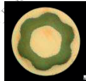
FIG. 5.9. ITER NbTi strand for ( \phi = 0.73\text{ mm} , WST) (Courtesy of the ITER Organization)
