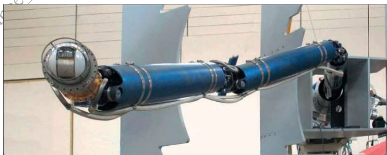
FIG. 11.29. The Articulated Inspection Arm inside the Tore-Supra mock-up [11.9].
