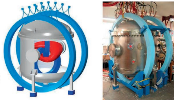
FIG.12.28 Cut-away view of Columbia Non-neutral Torus (CNT) [75] and the actual device.
