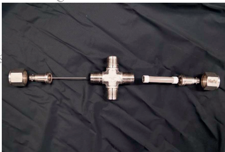
FIG. 10.16. Components of a small cross ionization chamber (active volume ~5 cm 3 ) for inline and real time measurements of the tritiated process gases used at TLK (courtesy F. Priester, KIT).
